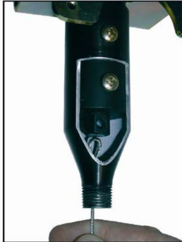
Photos show rocket cone 'cut-away' in order to show cable attachment more clearly.
